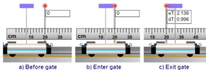
**Vector Gates.** Similarly to the photo gates, the vector gates use between 1 and 8 gates to take data. The vector gate data are snapshots of the various vectors as the cart passes the gate. To start the process, click Take Snapshots.
