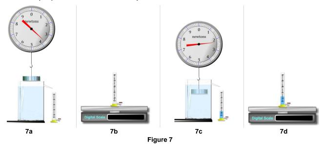
**Direct measurement of the buoyant force:** Weighing the aluminum disk in air (Fig. 7a) gives us W. Weighing it when submerged (Fig. 7c) gives us W. From our FBD (7e) we can see that
